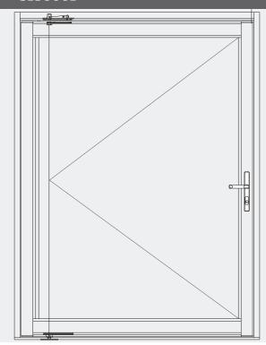
Series SI3000P thermally enhanced aluminum pivot doors can be used in commercial and residential applications. System design offers exceptional air, water, structural, and thermal performance in any condition. Multiple sill options and profile dimensions provide greater performance and design flexibility. Customization of product profiles, hardware, sills, panel size, and testing can be completed upon request.
